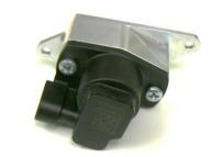
Slide sensor/adapter assembly onto the throttle shaft adapter. The sensor is spring loaded and will need to be rotated approximately 10 degrees against the spring to install the screws. A medium strength Loctite recommended on these screws.
