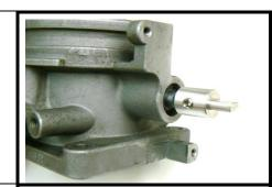
Install the sensor onto the adapter using 2 screws as shown. Tighten the screws
