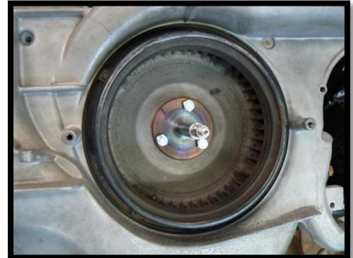
**Step 2** - Slide the bearing support over the trigger wheel shaft to the shoulder. Insert woodruff key into the trigger wheel shaft and install the trigger wheel assembly. Install washer and nut and tighten to 12 lb/ft.
